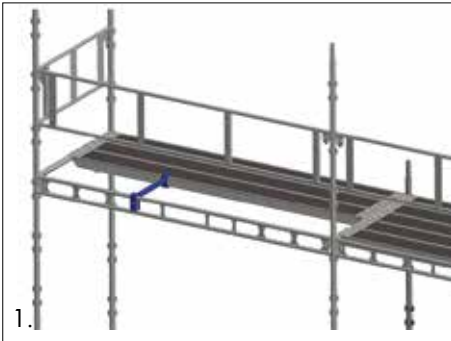
1. Remove 2x3050 steel decks and install a board to ledger bracket between the ledger beam and steel deck.
