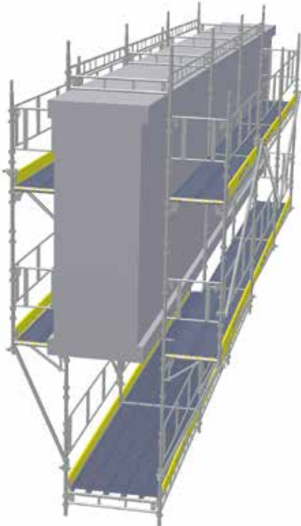
Example of section of scaffolding suspended from inverted beam.
