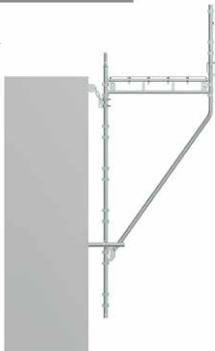
Example of suspended scaffolding with brackets.
