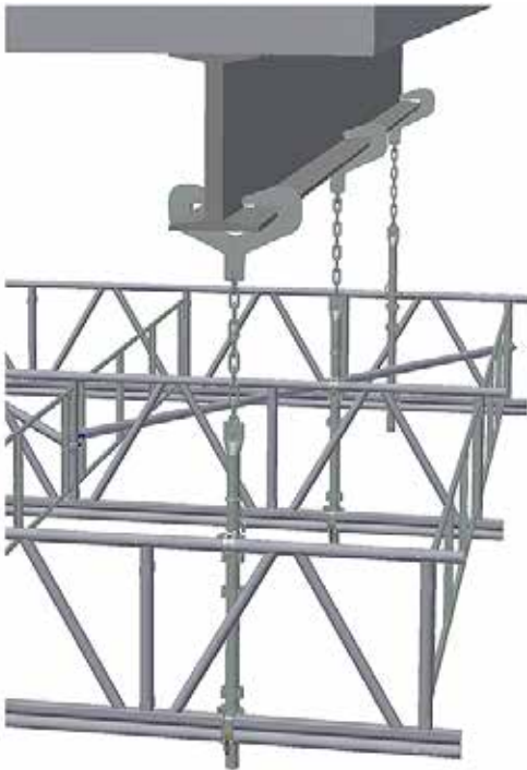
Example of wide suspended scaffolding with 750 AL lattice beams.
