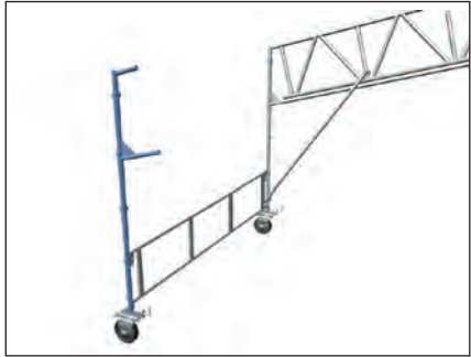
Figure 13 Fit Shelter Leg or Standard temporarily to stabilize the structure whilst construction of the 2nd half of truss is completed.
