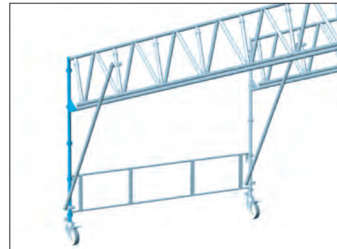
Figure 18 For 2nd half of this Truss repeat (8-12) but note to enable the permanent Shelter Leg to be fitted the temporary one must be removed.
