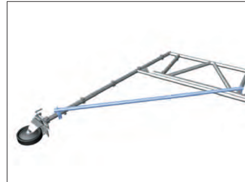
Figure 9 Locate the required Diagonal Brace (see page 7) onto Shelter Leg/Standard and on the vertical strut of the Aluminium Beam.
